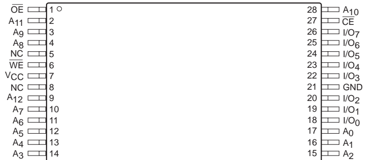
TSOP Top View (8mm x 13.4mm) (T13)
