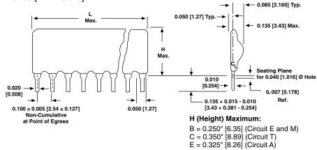
Pin #1 is extreme left-hand terminal on side with marking.
