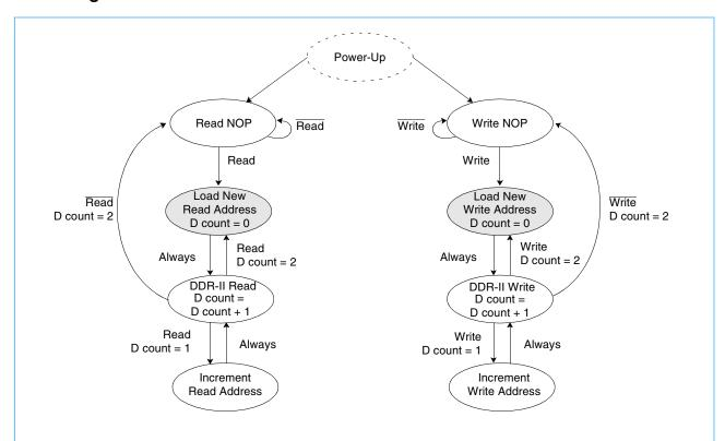
Notes: 1. Internal burst counter is fixed as four-bit linear; that is, when first address is A0+0, next internal burst addresses are A0+1, A0+2, and A0+3
