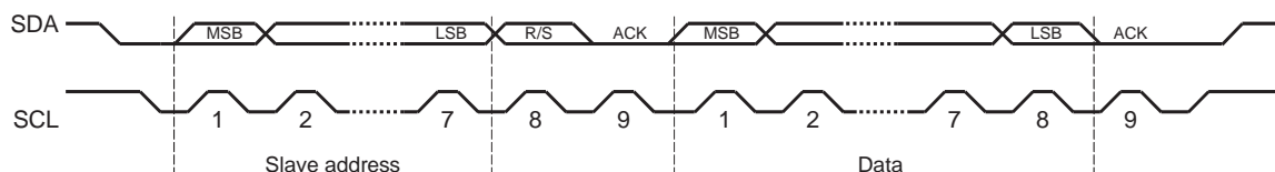
Figure 13-5. Complete Data Transfer with a 7-Bit Address
