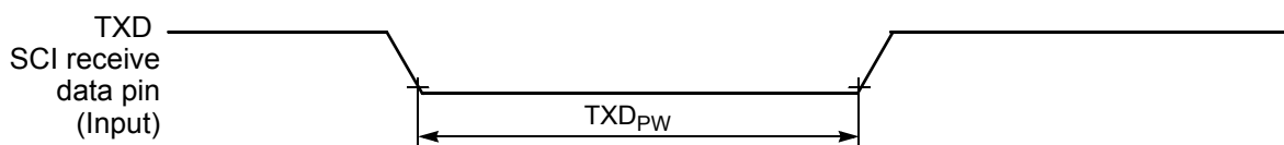
Figure 4-31 TXD Pulse Width
