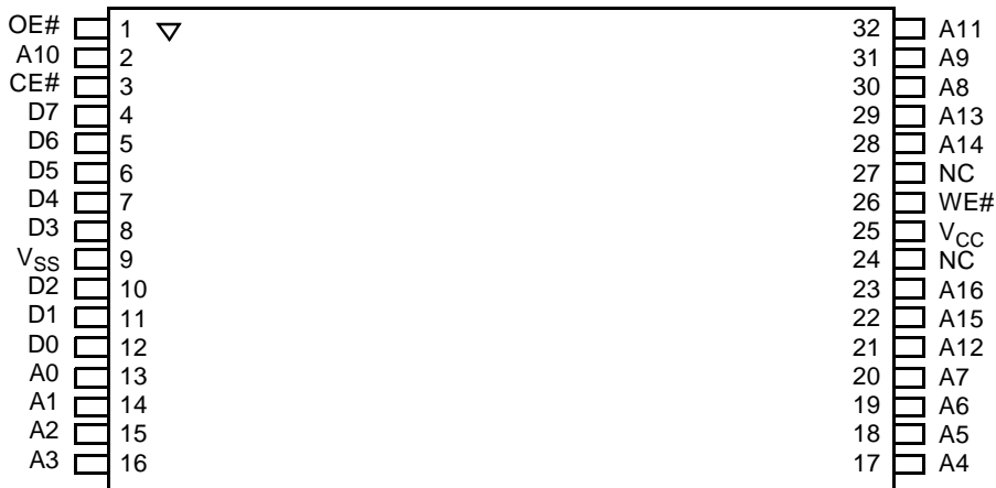
32-Pin TSOP—Reverse Pinout
