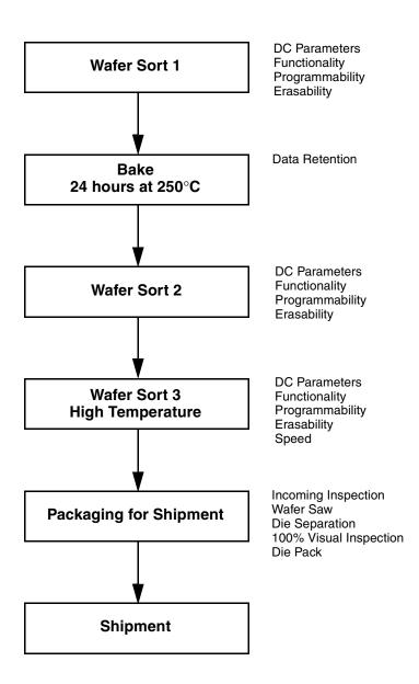
Figure 1. AMD KGD Product Test Flow
